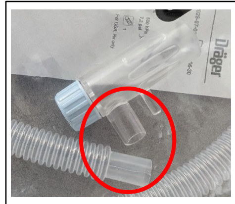
Fig. 2: Detached hose/ PEEP valve
