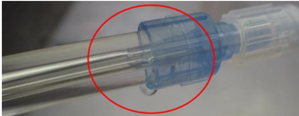
Figure 1: Example of L-70 leakage at tubing to return connector bond
