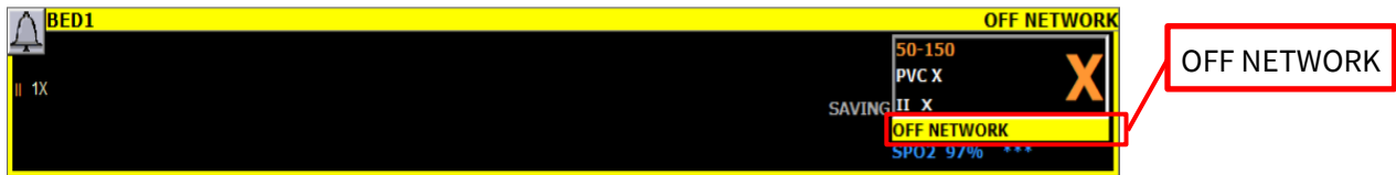
Figure 2. OFF NETWORK condition example in the Central Station Multi-Viewer window with audible and visual alarm indicators (bell icon and flashing title bar)
