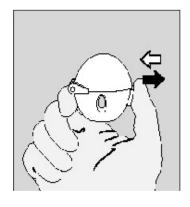
1. To release the dust cap press the piercing button completely in and let go.
