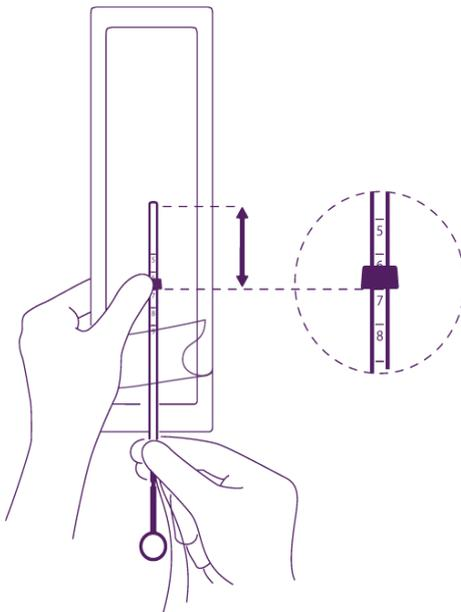
*Position the lower edge of the flange at the sounded value*
