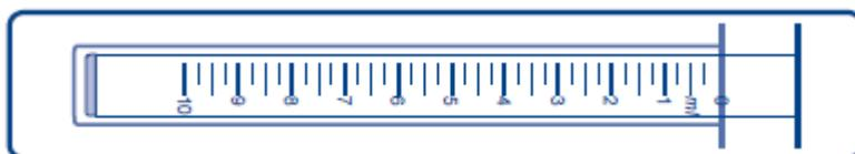
10 ml pipette, each numbered section is 1 ml and the smaller increments are 0.25 ml.
