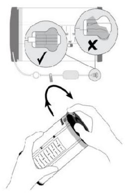
become visible in the window. Fluid flow can be seen upstream of the filter within seconds, but flow will stop until the nonvented cap is removed.
