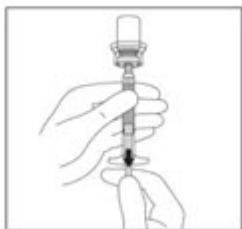
10. While holding the **white collar** of the syringe, unscrew the syringe from the SmartSite<sup>®</sup> Needle-Free Vial Access Device.
